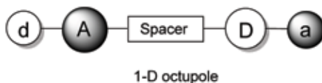
FIGURE 1. Schematic picture of a 1-D octupole ; ideally, a/A and d/D charge balance should be equal to 1/3 .
