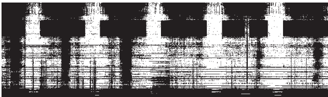
FIGURE 4 Usage of spectrum for 5 days, an instance of frequency band of Broadcasting TVI .
