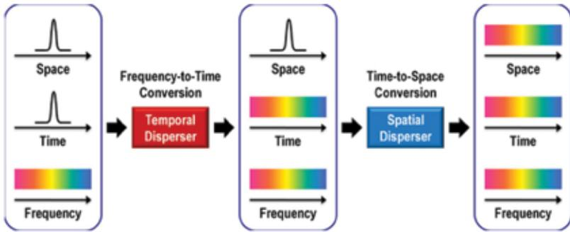
FIGURE 8 Schematic diagram of the pulse train frequency, time and space converter [105].
