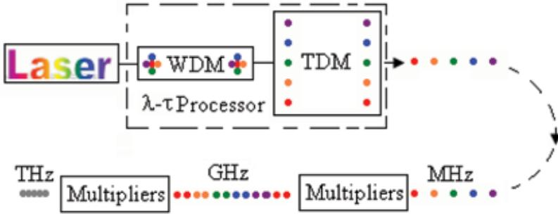
FIGURE 7 Schematic diagram of the wavelength and time multiplexed free-space pulse pinnate multiplier.
