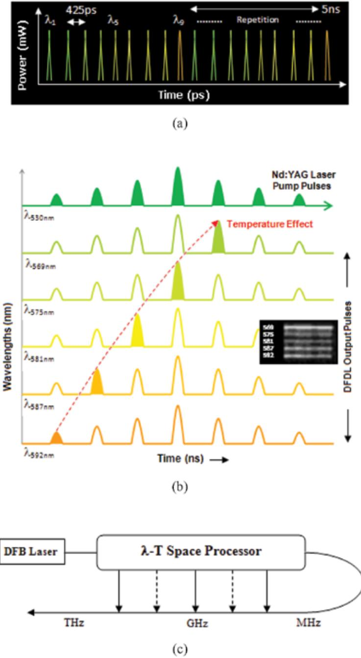
FIGURE 9 Wavelength, time and space processing and peak intensity wavelength shift for (a) WDM and TDM pulses, (b) Nd:YAG and distributed feed-back on dye laser (DFDL) pulses and (c) the experimental configuration for WTDM [109].
