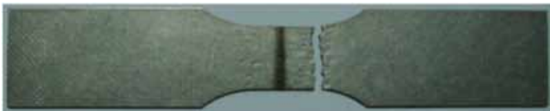
FIGURE 3 Photograph of the fractured tensile specimen for Sample #2.
