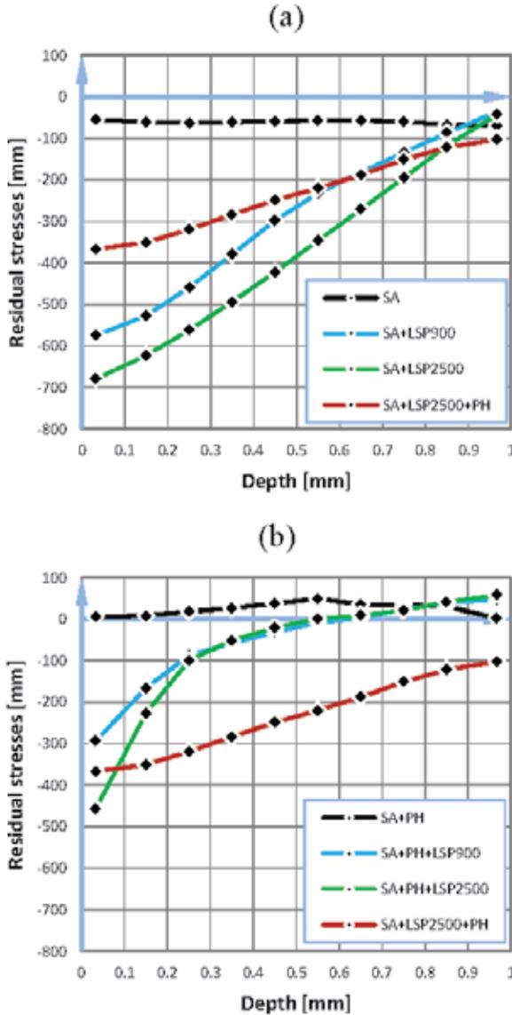
FIGURE 6 In-depth residual stress distribution before and after laser shock peening of maraging steel in the (A) solution-annealed condition and (B) precipitation-hardened condition using different laser pulse densities.
