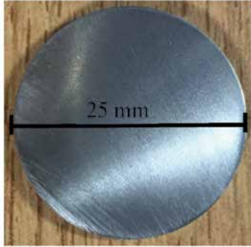
FIGURE 1 An optical image of Ti-6Al-7Nb alloy experimental sample.
