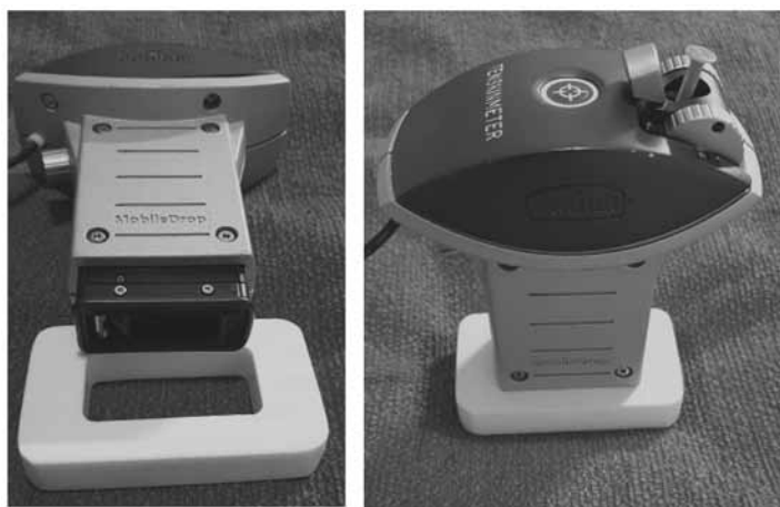
FIGURE 3 MobilDrop DSA2 (by Krüss - Hamburg – Germany) and Tensimeter with Teflon support for skin applications (Courtesy of Development Cooperation BAZH.I - NGO, Maserada Sul Piave, Treviso, Italy).
