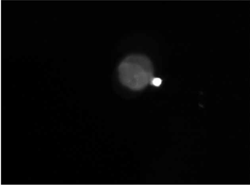
FIGURE 6 Image with contaminated cover slide.
