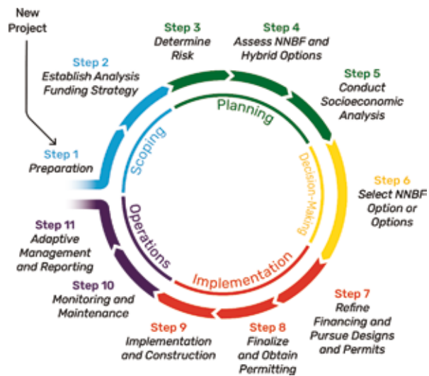
FIGURE 3 Framework for incorporation of natural and nature-based features (NNBF) in coastal projects (Graphics credit: Bridges et al., 2021, in press).
