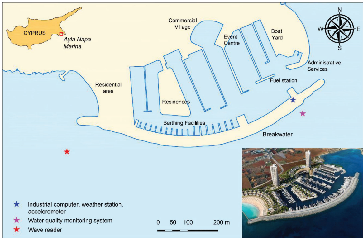
FIGURE 3 Ayia Napa Marina location map and layout of the monitoring system with inset aerial view.
